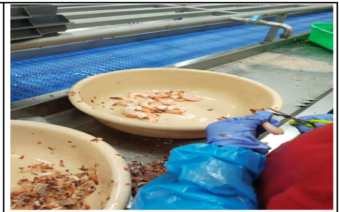
Black tail trimming in CIS checking table
