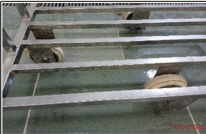
Trolley found formation of slime and it need to be cleaned properly.
