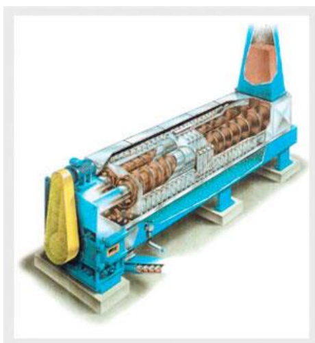
Figure 8 Twin screw press from Stord, The inlet is at the right side and outlet on the left (ATI Group, n.d.)
