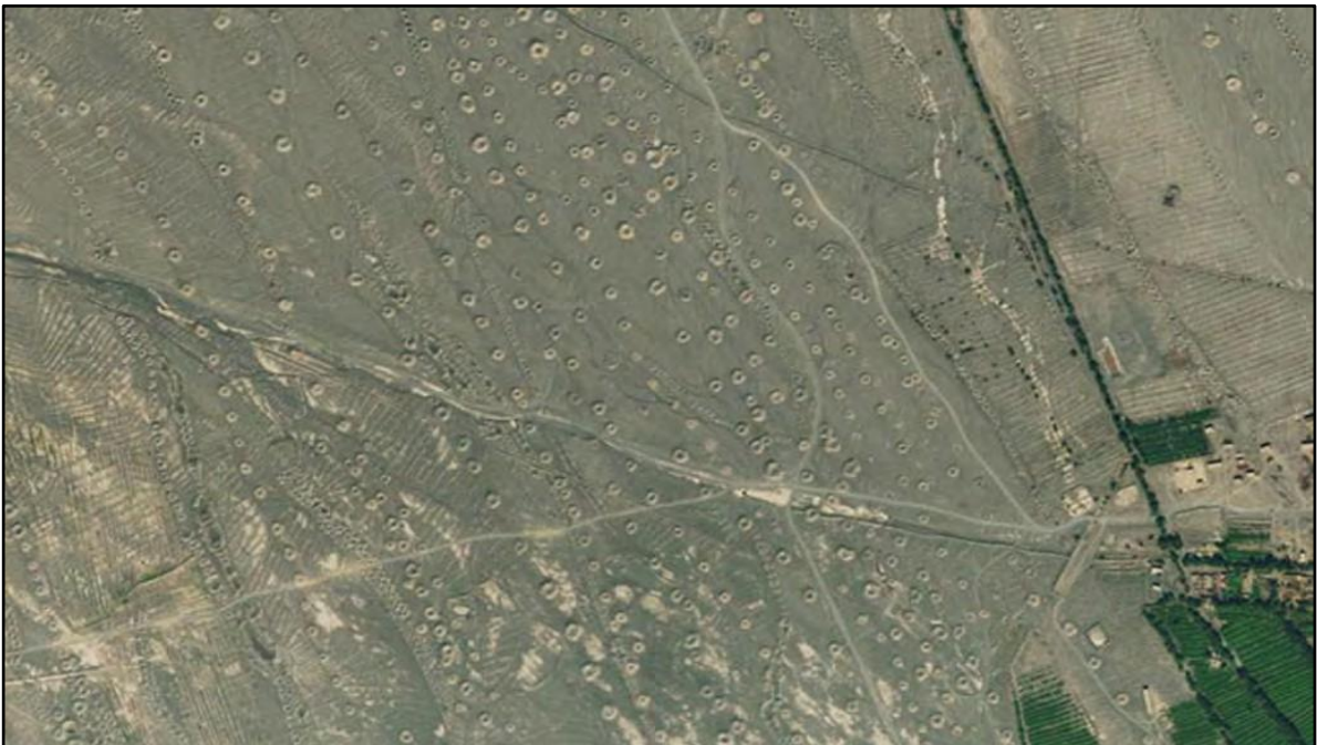
Aerial photograph: Course of karez tunnels in a barren mountain slope with "molehills" 3
